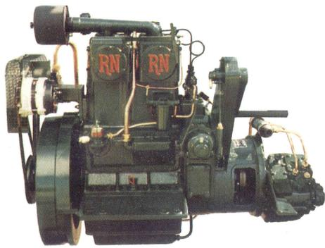
as much torque and have a maximum rpm of 5,000 or more. The power of a DM2 comes from its capacity, 2,628 cc for the two cylinders and the ingenious cylinder head design. Fuel consumption is around 2 to 3 hours of normal canal cruising from a gallon of fuel, or in metric terms 1 litre per hour. With only minor modifications to the fuel filter systems, it is possible to run the DM2 on low grade fuel, such as reclaimed lubricating oil or vegetable oils.
